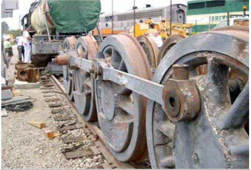
SCRVRHS volunteers from the Locomotive Workshop lend a hand on the Fillmore & Westerns' # 14 Baldwin 2-8-0 steam locomotive. Crews removed the springs that support the main wheels so that the F&W can send them out to have new sets made. Soon, the F&W plans to send the main wheels out to have machining done and new crown brasses made. The SCRVRHS Locomotive Workshop meets on the third Saturday of every month at 9:00 am, right after breakfast at Yanni's at 8:00 am. Interested? See Mark Aston.
